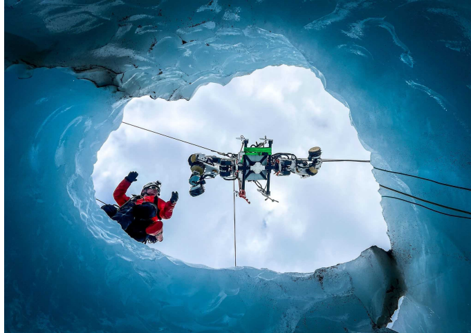
Figure 17. The EELS 1.5 robot being deployed into a moulin in Athabasca.
