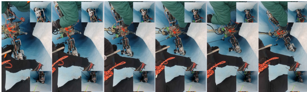
Figure 18. Successive frames showing the EELS 1.5 robot autonomously down-climbing into a moulin in Athabasca.
