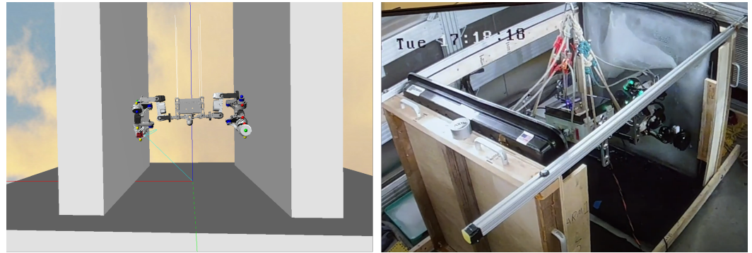
Figure 16. Left: view of the EELS 1.5 robot simulated within EELS-DARTS prior to executing its plan to engage contact with the wall and attempt to climb. White lines represent tethers. The red, green, and blue lines represent the inertial coordinate system. Right: image of the EELS 1.5 robot suspended within a vertical ice wall testbed inside a walk-in freezer lab at JPL.
