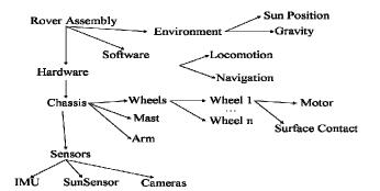
Fig. 9 A Rover Assembly Diagram. Related models within subsystems (e.g. a wheel motor, and surface contact model) can be grouped into a "wheel assembly." Assemblies are reusable and can be used in more than one simulation. This allows complex simulations to be built by choosing and connecting the desired assemblies together.
