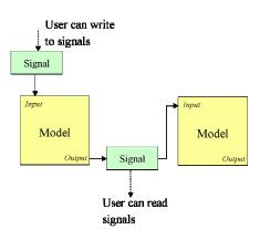
Fig.2 Data flow between models. In Dshell++, a model has user-defined *input* and *output* ports. Data is shared between models by tying a model's input port to another model's output port through a *signal* (basically a shared memory buffer). Users can peek or poke the signal data through the Dvar interface.
