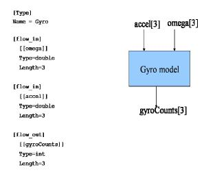
Fig. 8 Example of a model specification (.mdl) file. The user creates an .mdl file (a text file) to describe a model's inputs and outputs. For this example, the model simulates a hardware Gyroscope which has two inputs: the angular velocity (omega) and angular acceleration (accel). The output is an array of three integers which hold the gyro counts.
