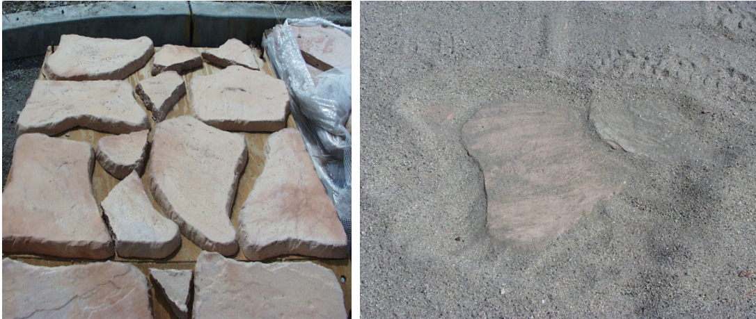
Figure 3. Underlying surface of MER tilt table with concrete paving stones glued to a plywood surface. The surface is then covered in sand to produce a mixed terrain.
