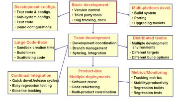
Fig. 1. Levels of software development environments ranging from individual developer/single product to distributed team with product-lines..
